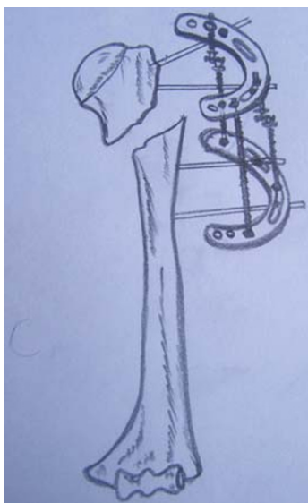
Fig. 5 Two arches were used for greater versatility. Hinges connecting the arches allowed translation and correction of angulation. The threaded rods were used to achieve distraction and final compression
