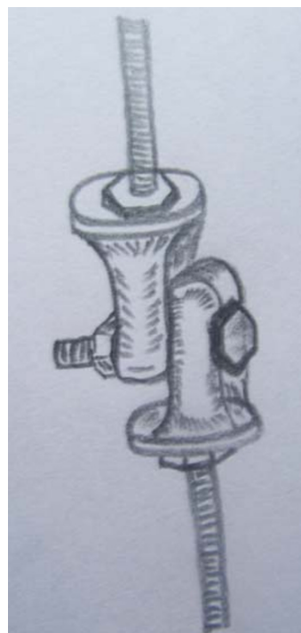
Fig. 6 This hinge assembly allows correction of angulation. Translation is achieved if additional hexagonal nuts are used
